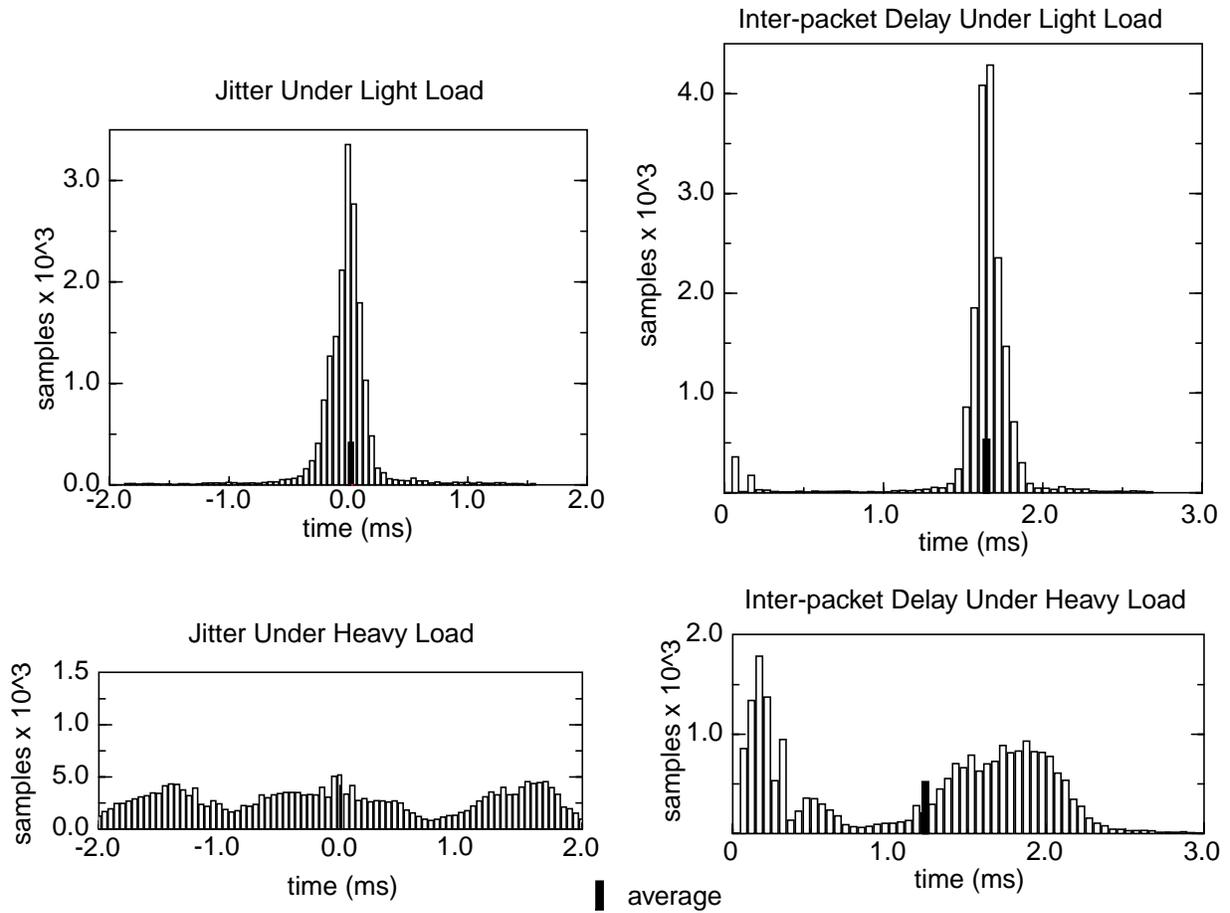
FIGURE 14. Example Jitter and Inter-packet Delay Histograms
